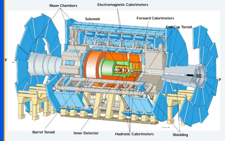
ATLAS is designed for a large discovery potential and for precision measurements. Experience and theoretical knowledge tell us that an experiment with this ambition should detect clean signals and perform accurate measurements of:
